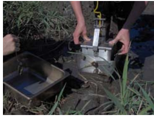
Sediment sample taken with a Ekman dredge
